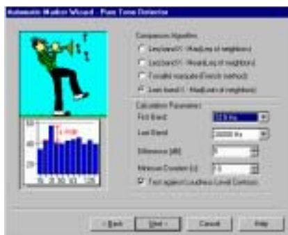
Fig. 6 Pure tone detection based on logged 1/3-octave spectra using one of the automatic Marker Wizards
